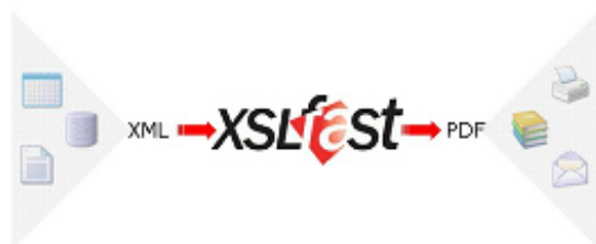
Illustration XSLfast is used to create layouts for XML data. These are available as XSL-FO-data for the automated processes in printable PDF format.
